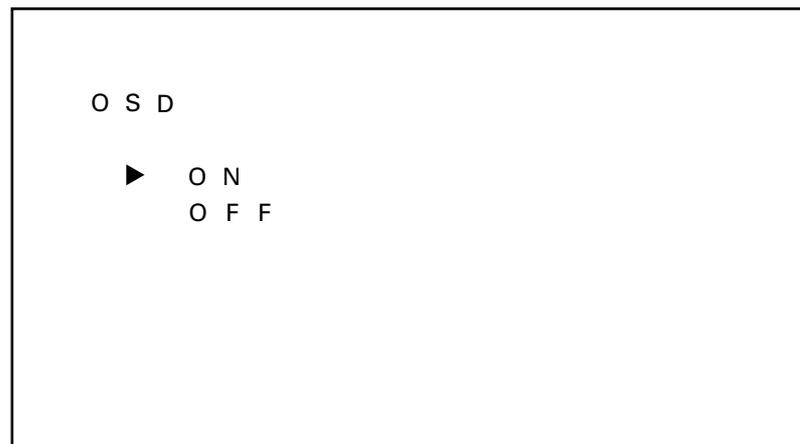
Operation is the same as with other input functions. With the remote control, use the ▲ and ∞ buttons to select the mode to be set, and confirm your selection with the SET button. With the operation panel, select the mode with the + and - buttons, then confirm your selection with the SET button.
