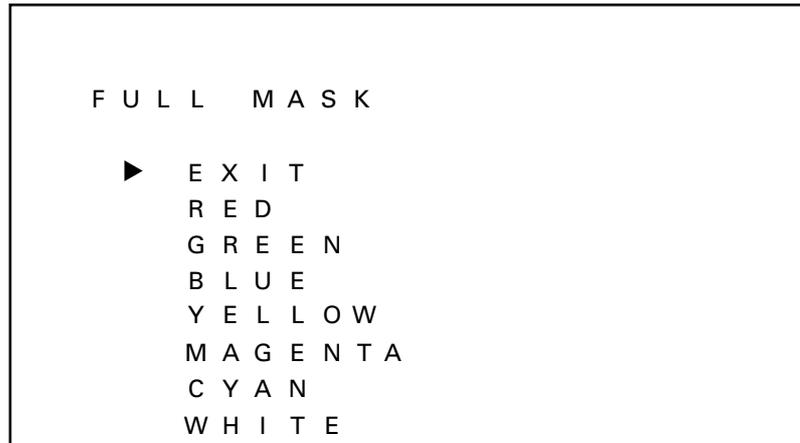
Operation is the same as with other input functions. With the remote control, use the ▲ and ∞ buttons to select the item to be set, and confirm your selection with the SET button. With the operation panel, select the item with the + and - buttons, then confirm your selection with the SET button.
